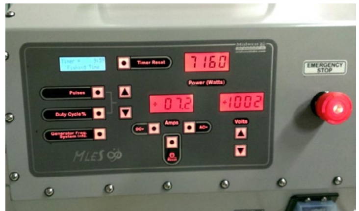
Close-up of MLES Infinity pulsator as used during actual test to shock mussels. Note the peak voltage was 1002 volts, and the applied power was over 7100 peak watts!
